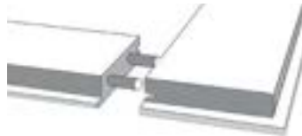
FRAME CONSTRUCTION construction elements connected using mounting pins
